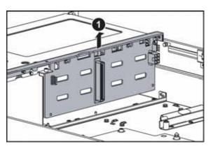
Pressing or pulling on any components on the backplane could result in damage to the backplane.
